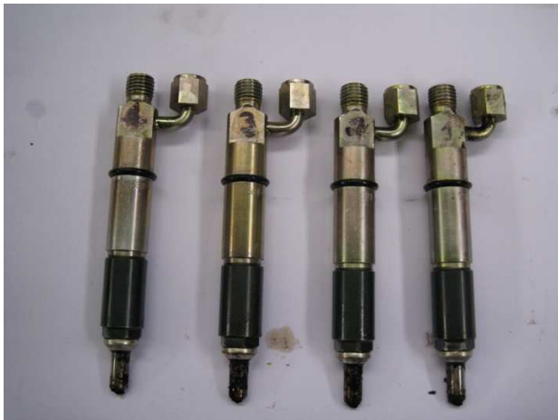
Fig.2. State of injector nozzle after overhaul.
