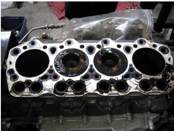
Fig.3. State of top side of pistons after overhaul.
