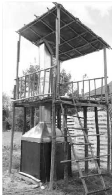
Fig. 3. Simulated open burning chamber.
