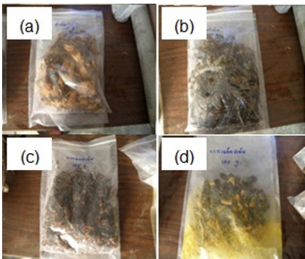
Fig. 2. The oil palm residues after soaking in 0.08% diluted sulfuric acid for 8 hours (a) Oil palm trunk. (b) Oil palm leaf. (c) Oil palm meal. (d) Oil palm seed meal.
