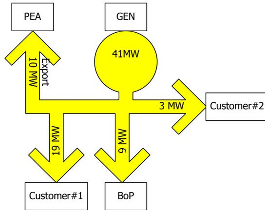
**Fig.5. Load flow diagram of a chosen SPP**
