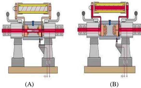
Fig.2. Current limiting devices by ABB [5], [6].
