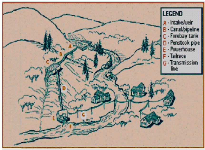
Fig. 1. Principal components of micro-hydro power systems
