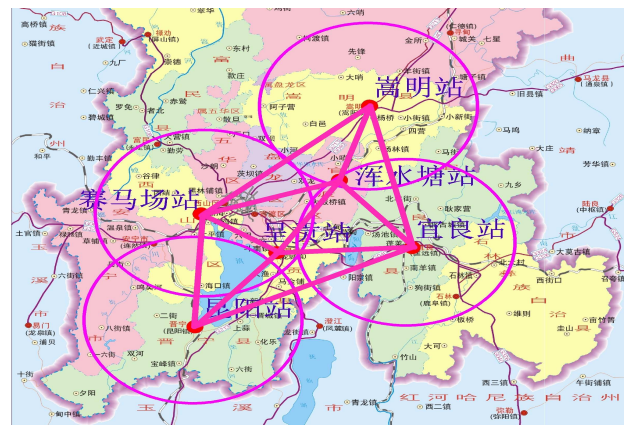
Fig. 3. The structure of Kunming city CORS.
