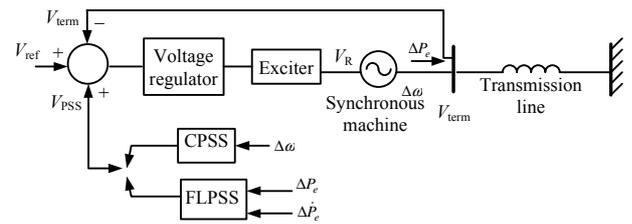
Fig.11. Single-machine infinite-bus system with CPSS and FLPSS.
