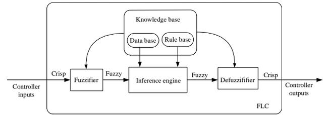
**Fig. 5.** Schematic diagram of the FLC building blocks
