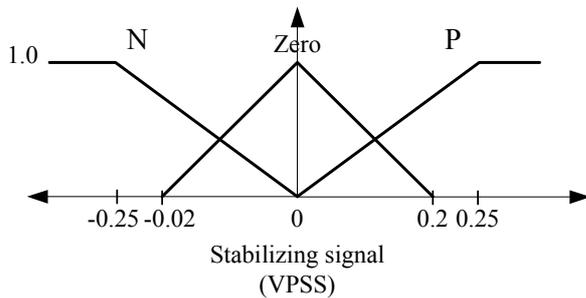
Fig.9. Three fuzzy sets of stabilizing signal (VPSS).
