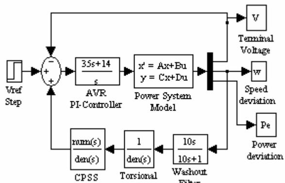
Fig.2. Simulink diagram of conventional power system stabilizer.
