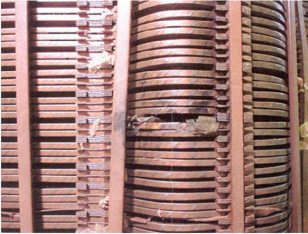
Fig. 12. Buckling of coil with leakage reactance -3.4%.
