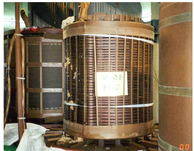
Fig. 11. Buckling of coil with leakage reactance -4.6%.
