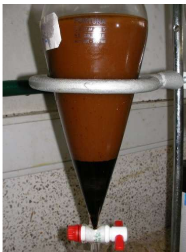
Fig. 5. Product from step 1 (acid esterification) during the separation process.
