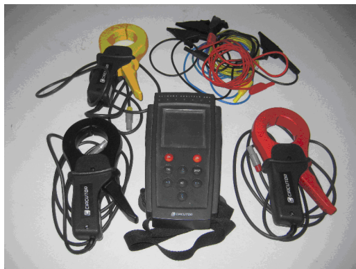
Fig. 6. Electrical network analyzer.
