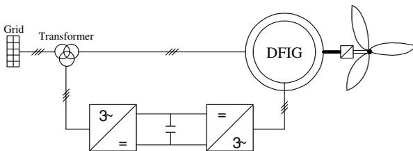
Fig. 2. Block diagram of doubly fed induction generator wind turbine system.
