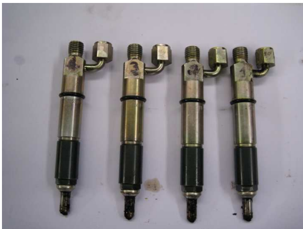
Fig.2. State of injector nozzle after overhaul.
