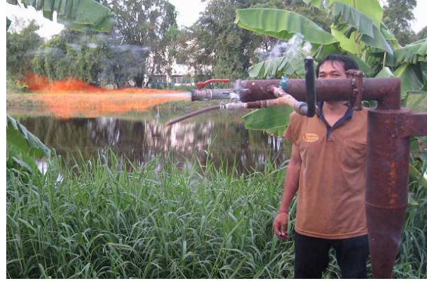
Fig. 4. Firing of the obtained producer gas.
