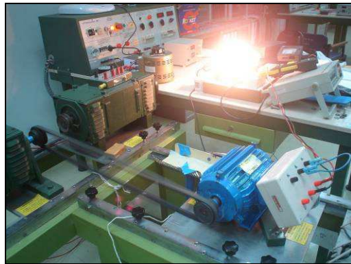
Fig. 7. Testing station of low speed generator prototype with the electrical load.
