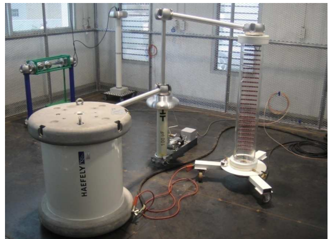
Fig. 8. Testing Circuit of Rated Voltage 100 kV rms
