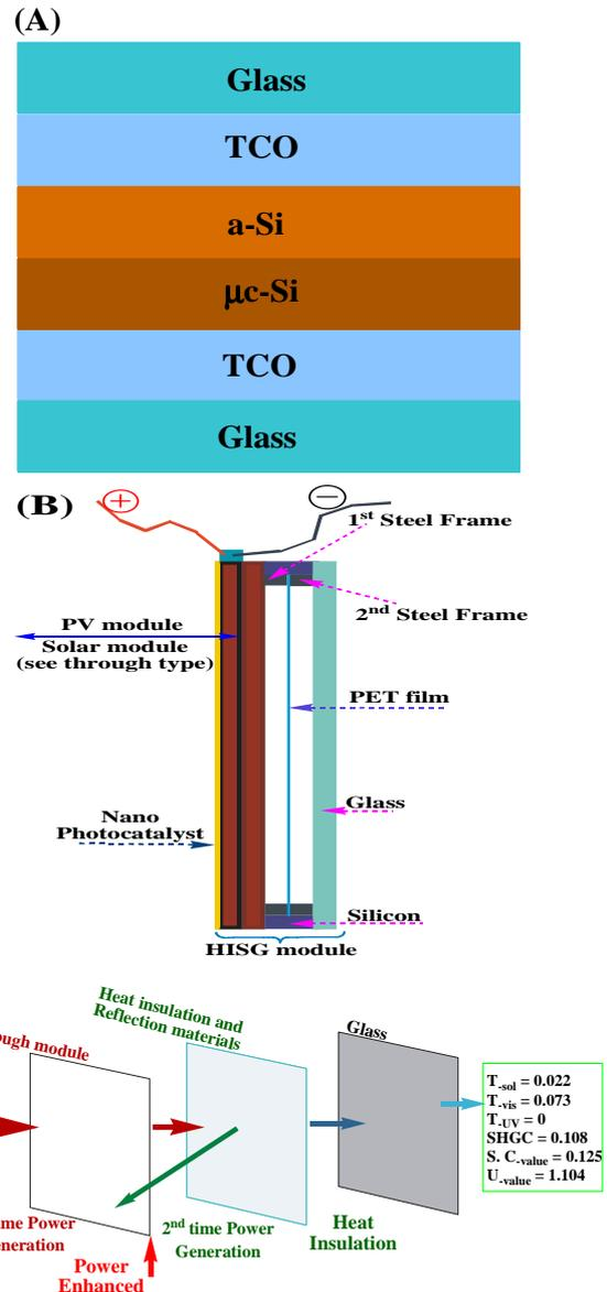
Fig. 1. Structures of (A) original PV module and (B) HISG module (thickness ~28 mm), and (C) Scheme about function theory of HISG ( $T_{sol}$  is the solar transmittance,  $T_{vis}$  is the visible light transmittance,  $T_{UV}$  is the UV transmittance, SHGC is the solar heat gain coefficient, S.C. is the shading coefficient, and U value is the thermal transmittance of HISG) [16].
