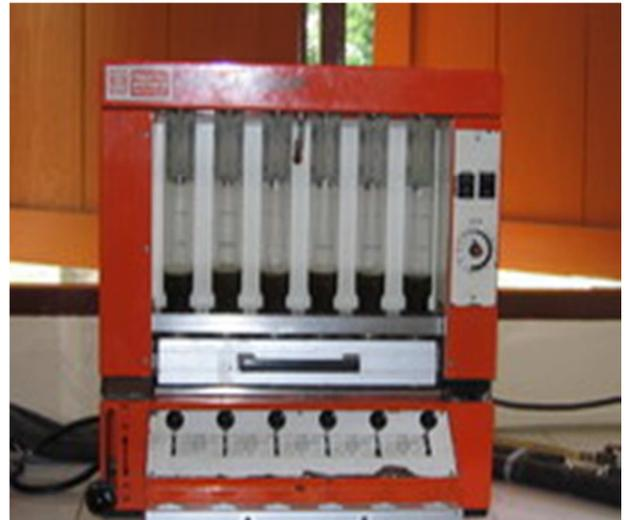
Fig 8. Analysis of % ADF as ADF testing method.
