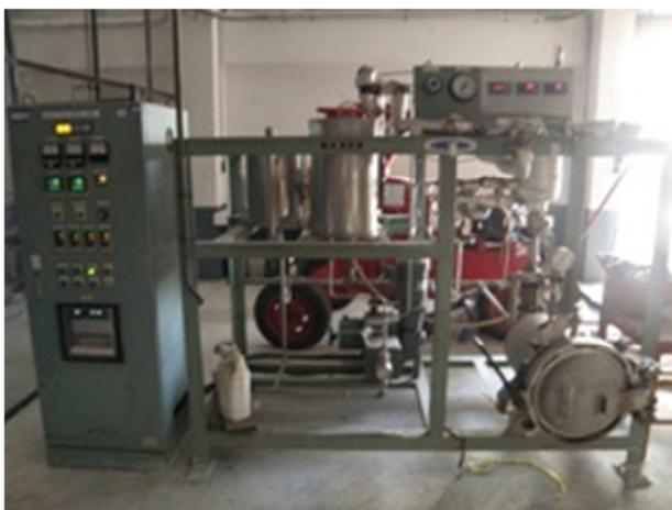
Fig 3. The steam explosion machine.
