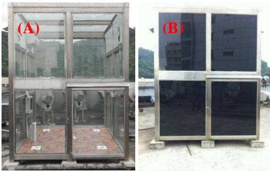
Fig. 9. Outside appearance of experimental houses: (A) Ordinary House (using Normal glass) and (B) Heat Insulation Solar House (using HISG).
