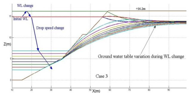
Fig. 7. Result of ground water variation (case 3)
