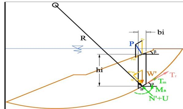
Fig. 2. Free body diagram of slip surface and slice with no inter-slice forces (Fellenius method).
