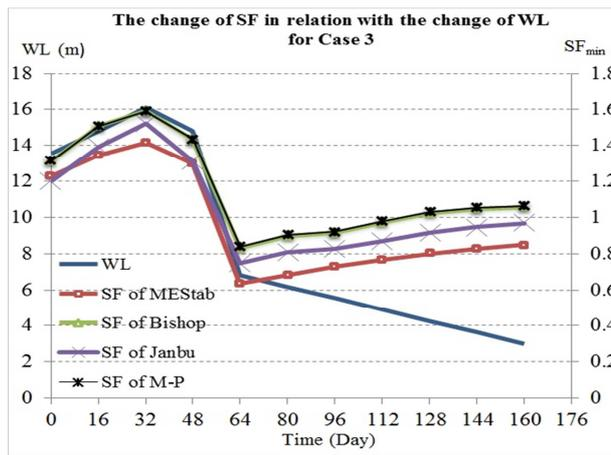
Fig.10.  $SF_{min}$  calculated by MESTab and Slope-W for Case 3.  $min[SF_{min}]=0.634$
