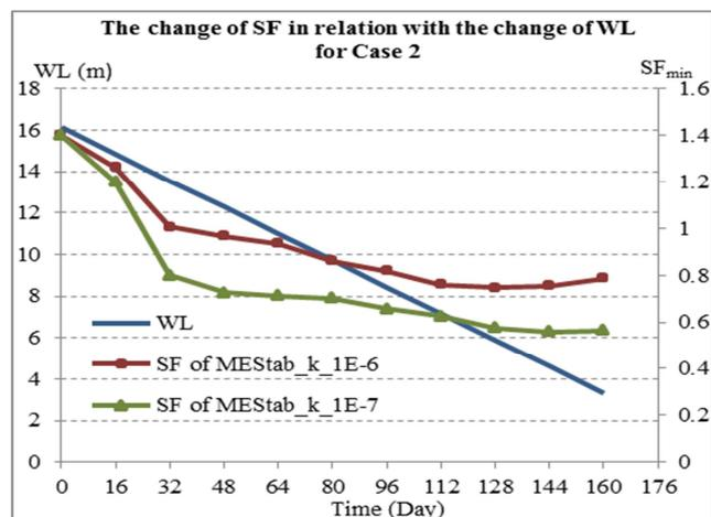
Fig.12. Influence of soil permeability on  $SF_{min}$ , Case 2
