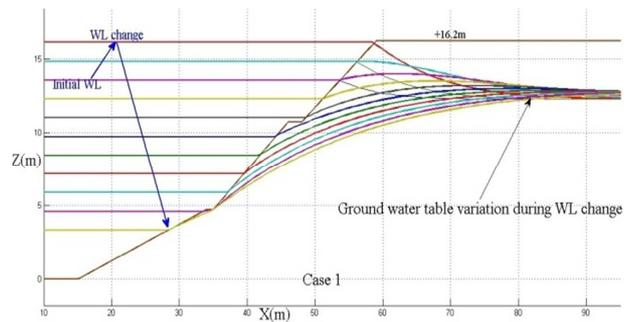
Fig. 5. Result of ground water variation (Case 1).
