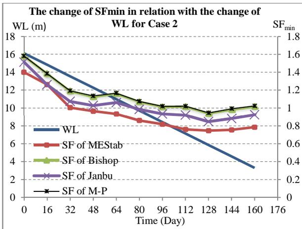
Fig.9.  $SF_{min}$  calculated by MESTab and Slope-W for Case 2.  $min[SF_{min}]=0.746$
