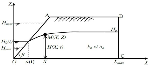
Fig. 1. Notations of ground water model.
