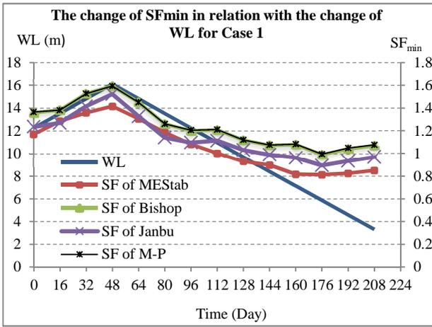
Fig.8.  $SF_{min}$  calculated by MESTab and Slope-W for Case 1.  $min[SF_{min}]=0.814$
