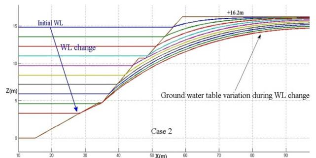
Fig. 6. Result of ground water variation (Case 2).
