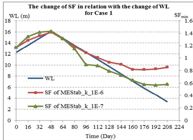
Fig.11. Influence of soil permeability on  $SF_{min}$ , Case 1
