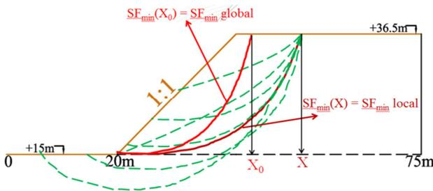
Fig.14.  $SF_{min}$  of a river bank
