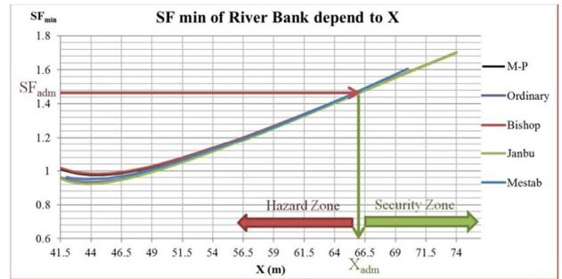
Fig.15. Definition of hazard and security zones
