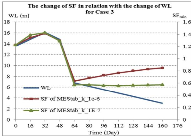
Fig. 13. Influence of soil permeability on  $SF_{min}$ , Case 3
