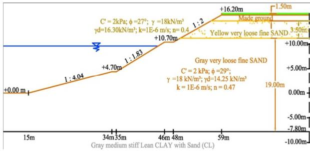
Fig.3. Mekong River bank geometry and soil properties (Kampong Cham)
