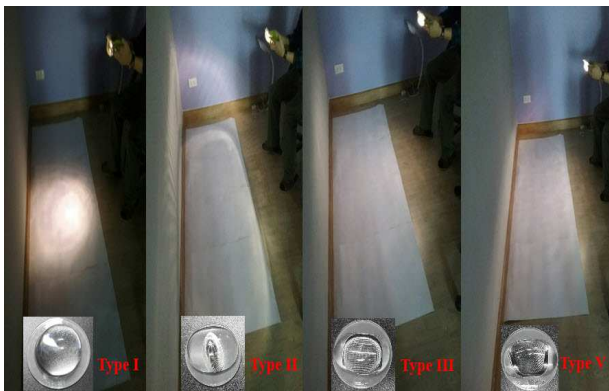
Fig. 8. Light distribution of big lens types (Type I: O shape, Type II: I shape, Type III: oval shape, Type V: U shape).
