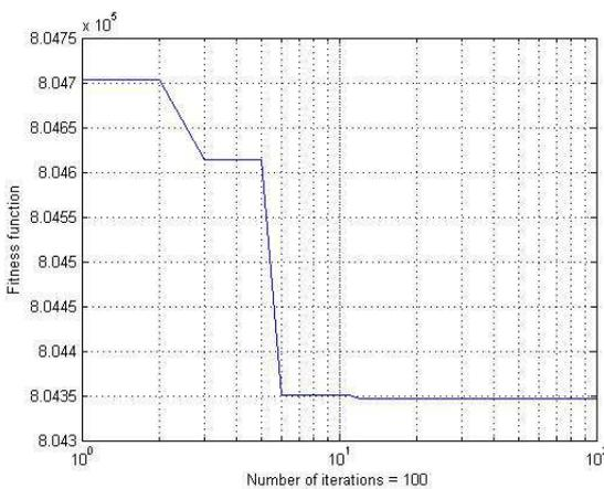
Fig. 4. The convergence characteristic of CSA for the IEEE 118 bus system.
