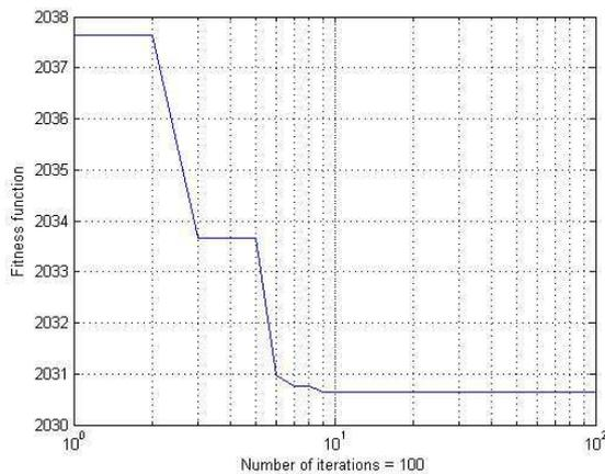
**Fig. 2. The convergence characteristic of CSA for the IEEE 30 bus system.**
