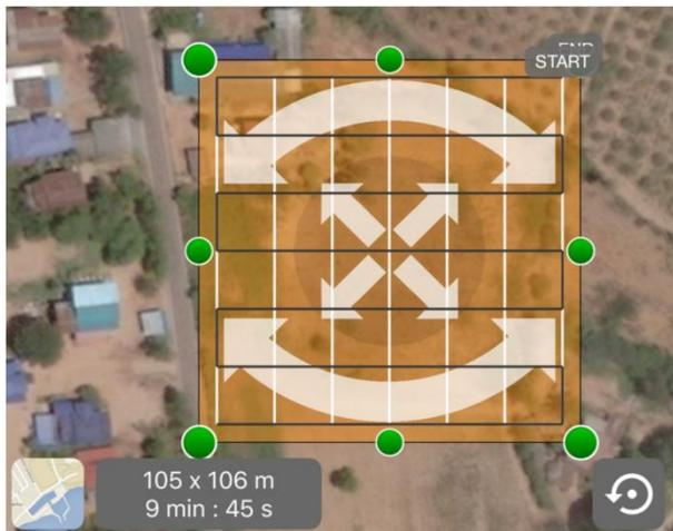
Fig. 1. UAV flying pattern for taking photos.
