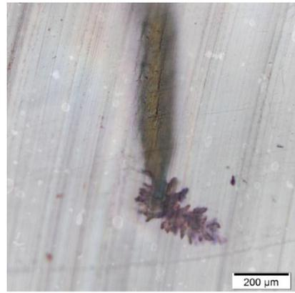
Fig.27. Water treeing in palm-crack shape.
