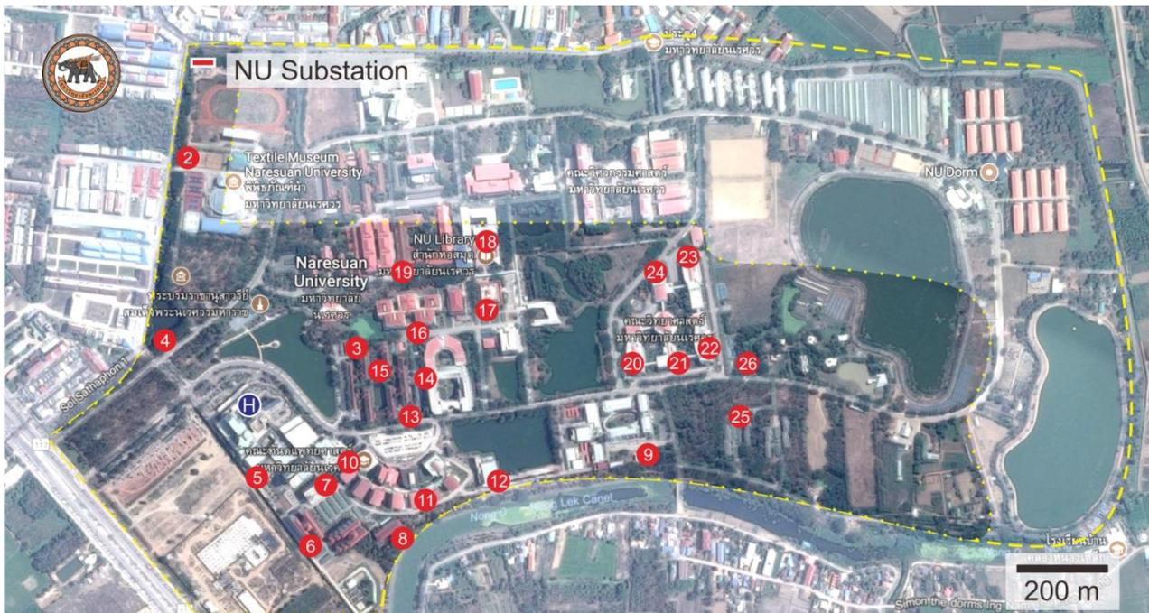
Fig. 1 Map of Naresuan university (NU). The NU substation and the location of the transformers of the feeder no. 1 are marked as a red rectangle and red circles, respectively. The bus numbers are labeled by the numbers. The location of NU hospital is marked by H.
