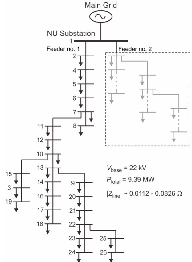
Fig. 2 Single line diagram of the NU power system.
