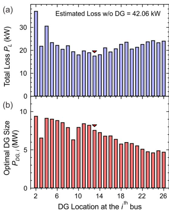
**Fig. 3 (a) Total transmission loss and (b) the optimal DG size when the single DG with optimal DG size is installed at various bus locations**
