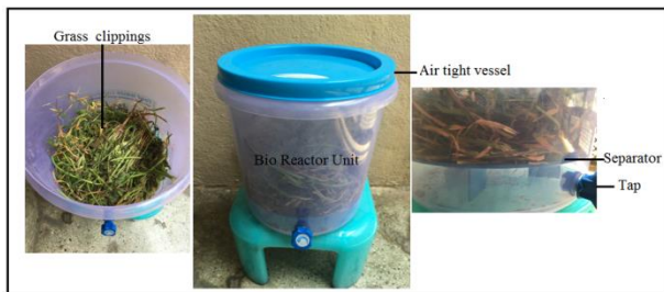
Fig. 13 The separator (Blue color), Tap (Blue color), grass clippings, the airtight vessel and the bioreactor unit experimental setup.
