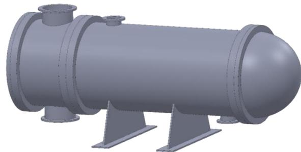
Fig. 2. ST HTX with a plate holding a continuous spiral used in the analysis.
