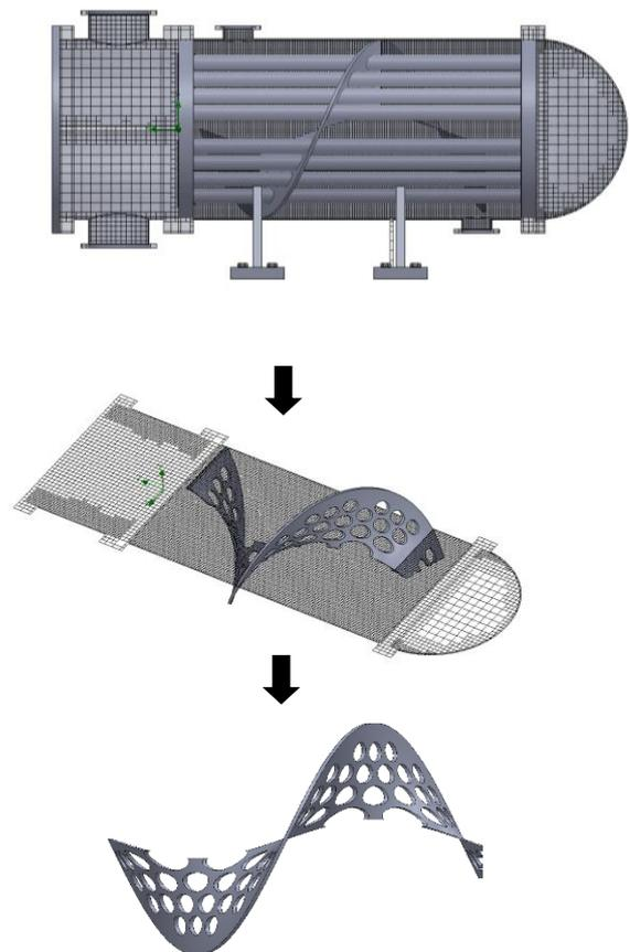
Fig. 4. The geometry and generated grid.
