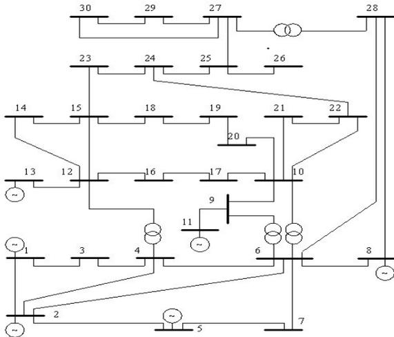
Fig 3. IEEE 30 Buses Test System.
