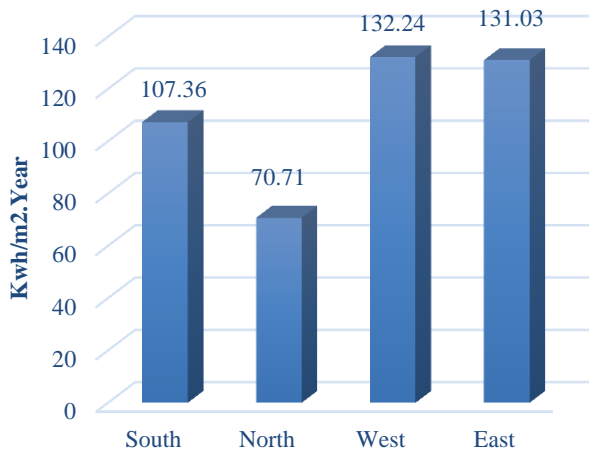
Fig. 4. The annually average energy generated from solar panels in the building sides ( K_{s,j} ).
