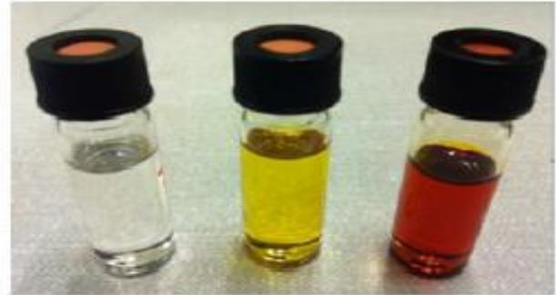
Fig. 1. Aging oil considering IEC611125- fresh oil (bright white), after one-week aging (dark yellow), after 2 weeks aging (dark brown) [21]
