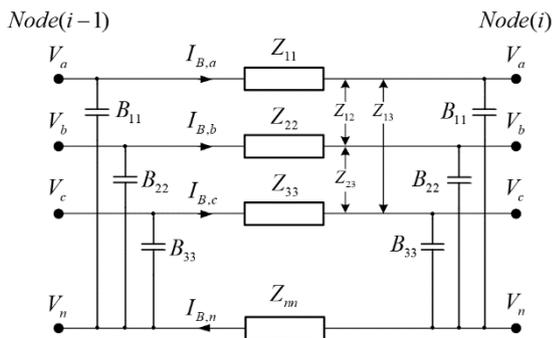
Fig. 2: Three phase transmission line model [7].
