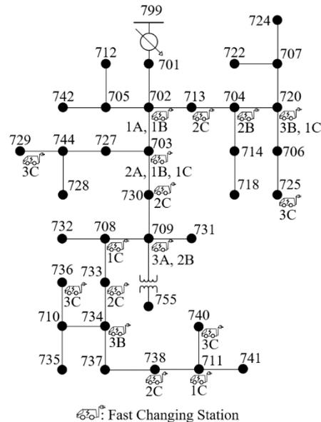
**Fig. 4: IEEE 37 bus connected with FCS.**
