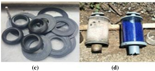
(a) Rubber Gasket Deteriorated (b) Less Dielectric of Oil (c) Rubber Shield Deteriorated (d) Silica Gel Deteriorated
