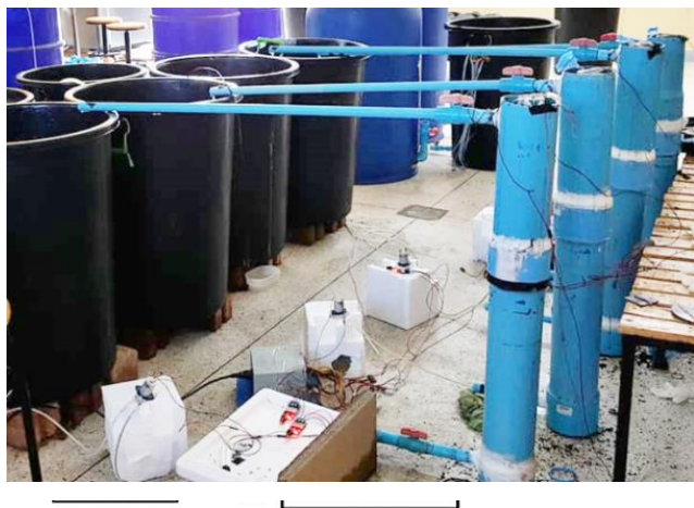
Fig. 1. Four membrane-less, single chamber BMFCs used in this study.
