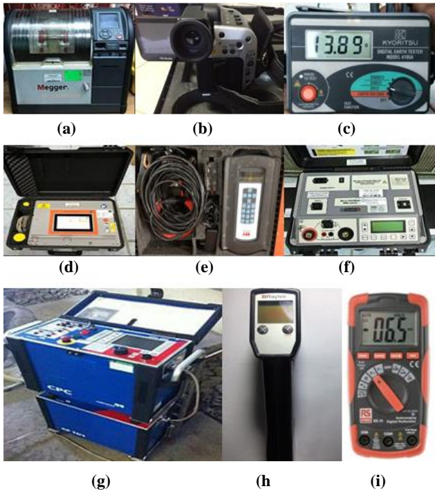
(a) Test Oil Maker (b) Thermo Scan (c) Earth Ground Tester (d) SF 6 analyzer (e) Capacitance meter (f) Micro ohm meter (g) Transformer test (h) Infrared Tester (i) Multi meter
