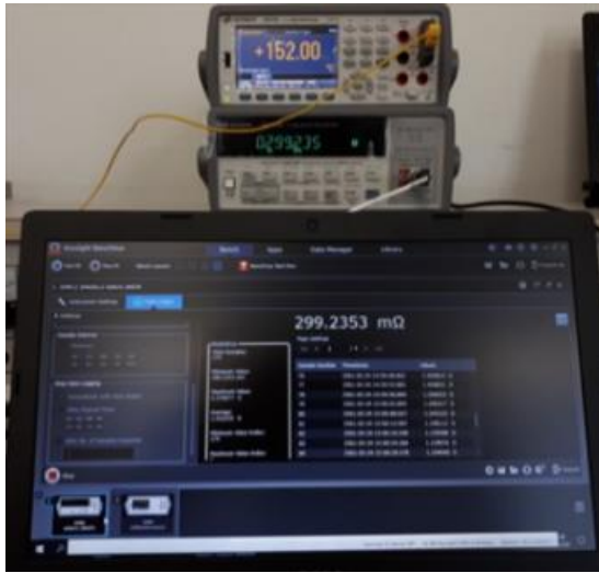
Fig. 5. The DMM and the MODM while monitoring and testing data storages.
