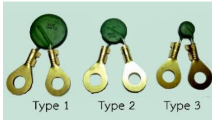
Fig. 2. The three NTC thermistor candidates.
