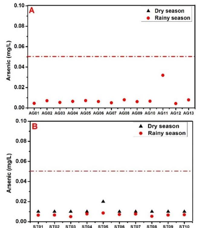
Fig. 9. Total Arsenic Concentrations of Water in (A) An Giang Prov. and (B) Soc Trang Prov.
