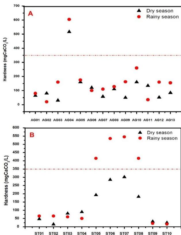
Fig. 10. Hardness of Domestic Water in (A) An Giang Prov. and (B) Soc Trang Prov.
