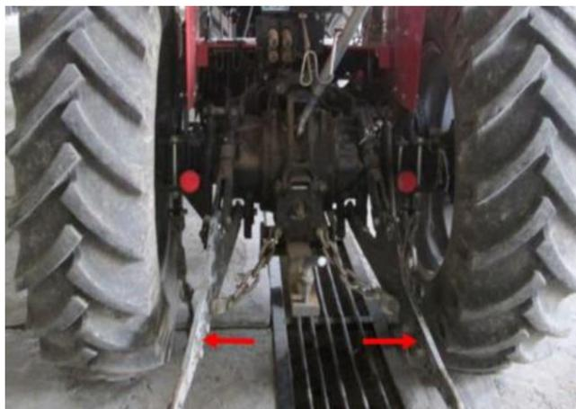
Fig. 5. Installation area of the lower extension arm to the tractor.
