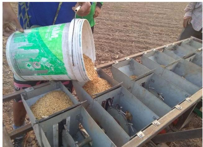
**Fig. 13. Vertical seed swivels disc with sowing machine.**
