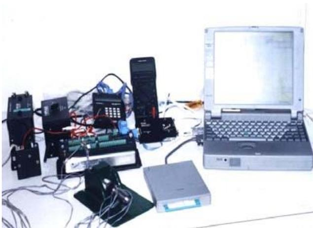
Fig. 14. Data MT-250D and acquisition system.
