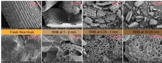
**Fig. 4. Morphology of rice husk and rice husk biochar (RHB) at different sizes at two magnifications; 100x (top) and 1000x (bottom) by FESEM-Eds.**
