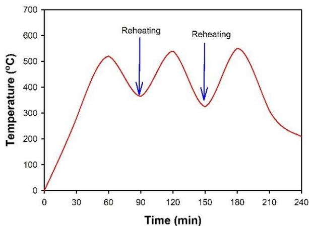
Fig. 2 Pyrolysis temperature of RHB production in biochar kiln.
