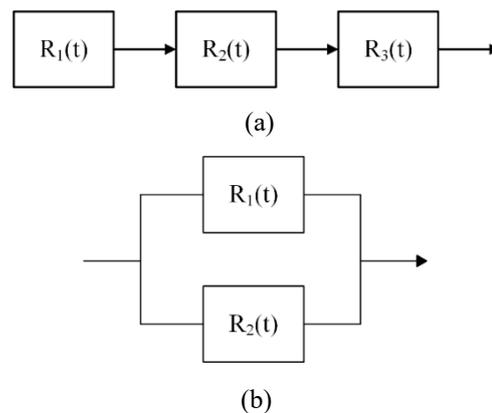
**Fig. 2 (a) series connected blocks (b) parallel connected blocks.**
