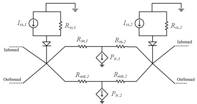
**Fig. 1. The equivalent circuit of DC traction power supply.**
