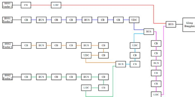
Fig. 7 Reliability block diagram of Klong Bangphai traction substation.
