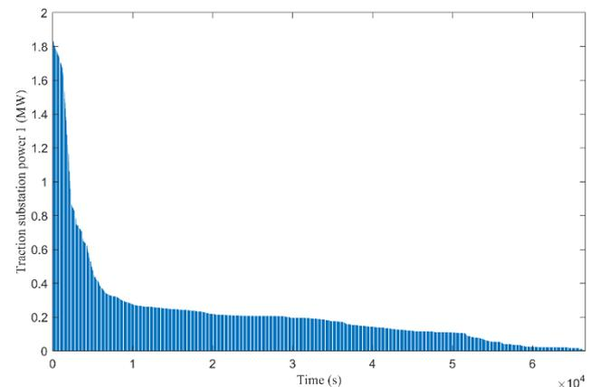
**Fig. 6 Load duration curve of traction substation at Klong Bang Phai.**
