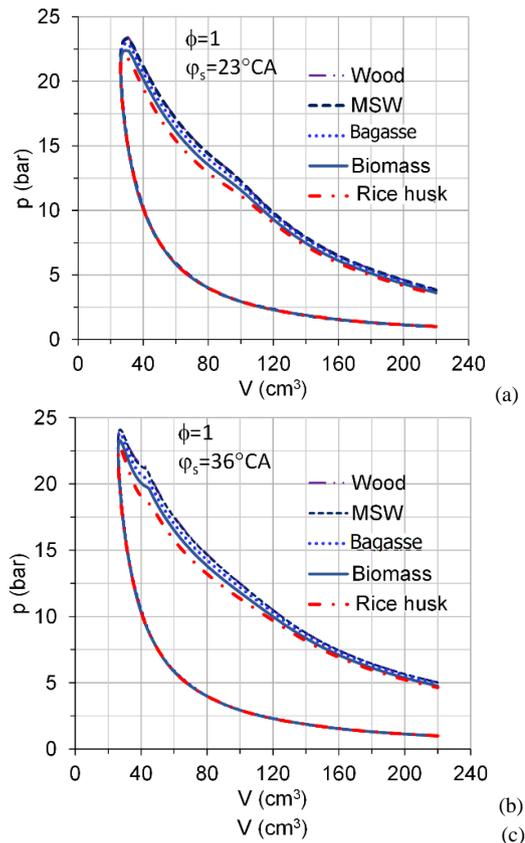
**Fig. 3.** Effects of equivalence ratio and advanced ignition angle on indicative work diagram of the engine fueled with syngas obtained from gasification of different biomass
