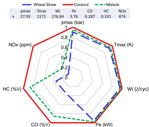
Fig. 7. Comparison of combustion characteristics when syngas powered engine obtained from separate RDF and from the mixture of coconut shell and wheat straw RDF.
