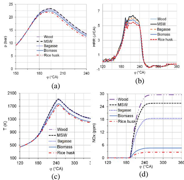
**Fig. 1.** Effect of syngas on variation of pressure (a), heat release rate (b), temperature (c) and NOx (d) according to crankshaft angle ( $n=3000$  rpm,  $\phi=1$ ,  $\phi_s=30^\circ\text{CA}$ ).
