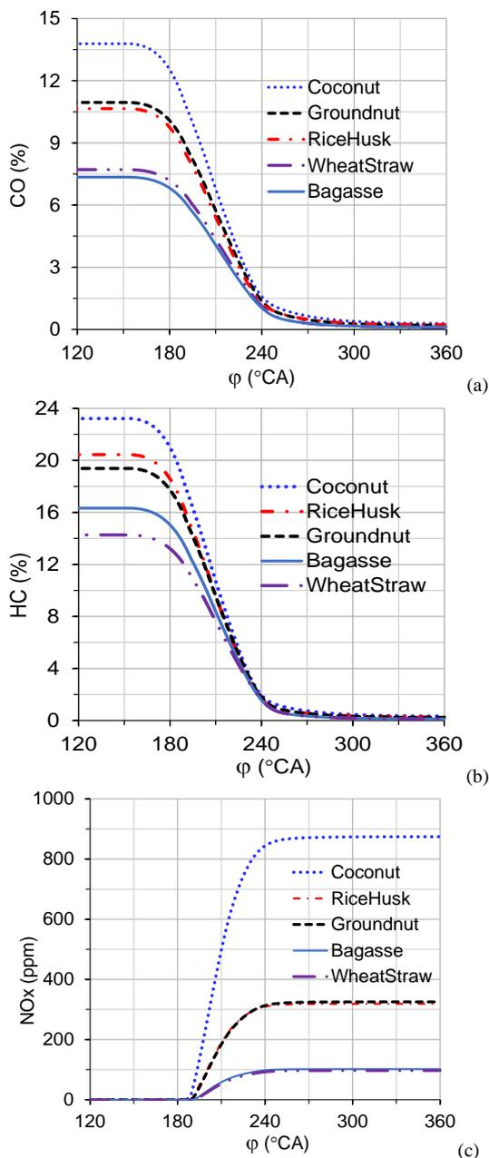
Fig. 5. Variations of CO (a), HC(b), NOx(c) concentration with crankshaft angle when the engine runs at 3000 rpm,  $\phi = 1$ ,  $\phi_s = 30^\circ\text{CA}$  on the RDF-syngas received from different kinds of raw materials.
