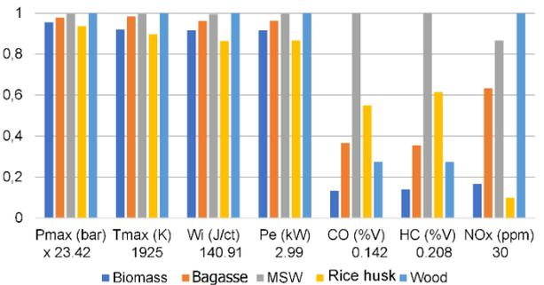
**Fig. 2.** Comparison of combustion characteristics of the engine fueled with syngas from different types of biomasses
