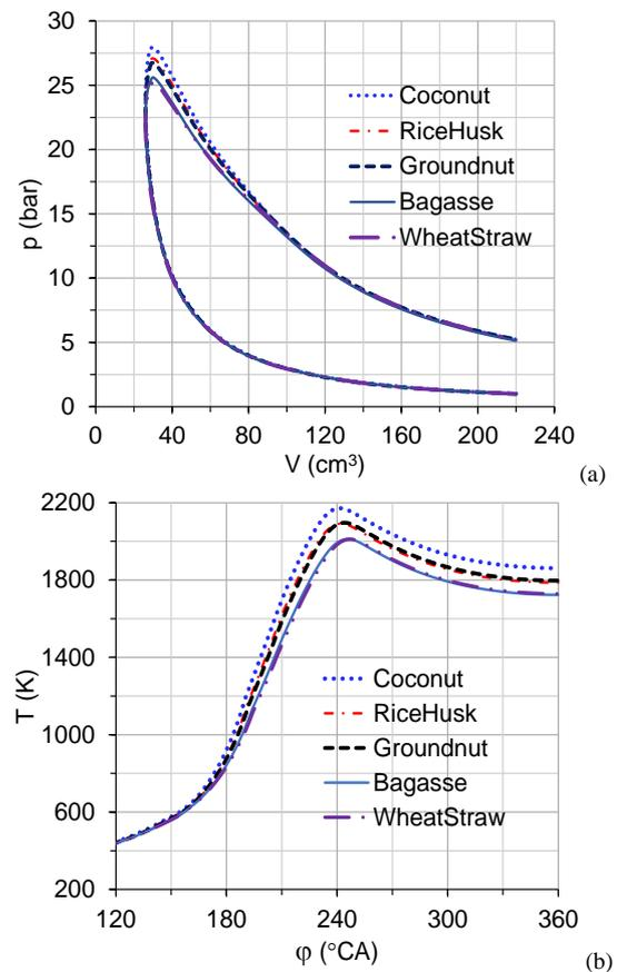
**Fig. 4. Effects of RDF-syngas received from different kinds of raw materials on indicative work diagram (a) and on variation of temperature according to crankshaft angle (b) when the engine operates at 3000 rpm,  $\phi=1$ ,  $\phi_s=30^\circ\text{CA}$ .**
