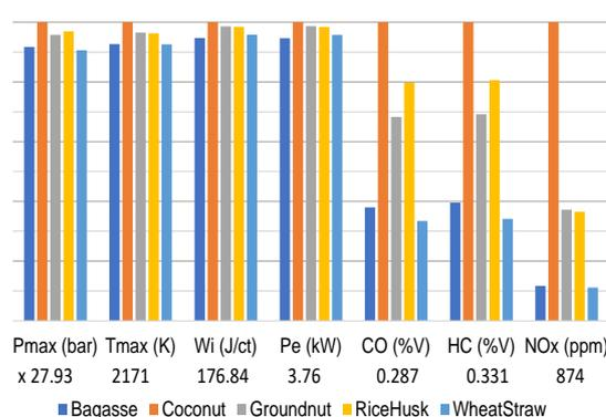
Fig. 6. Comparison of combustion characteristics of the engine fueled with syngas from the gasification of different RDF feedstocks.
