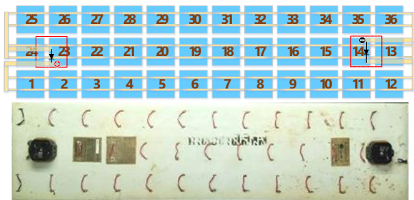
Fig.3. Diagram of cells on PV module 53 Wp.
