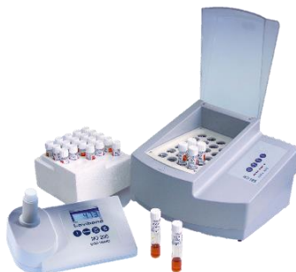
Fig.5. Chemical oxygen demand (COD) analyzer.
