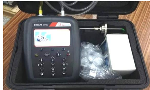
Fig.7. Biogas composition measurement analyzer.
