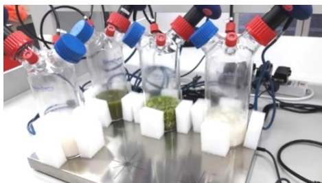
Fig.6. Biochemical methane potential (BMP) analyzer.
