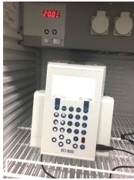
Fig.4. Biochemical oxygen demand (BOD) analyzer.
