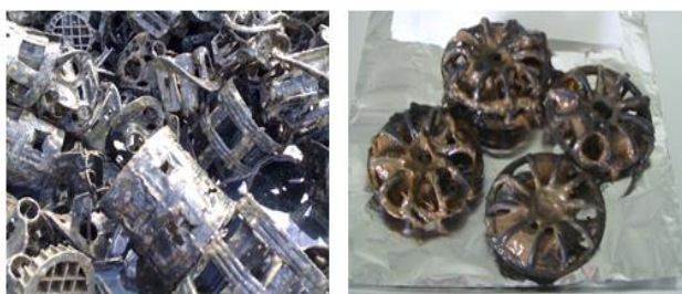
Fig. 2. Packing media used in the packed bed absorbers of STR20 industry.
