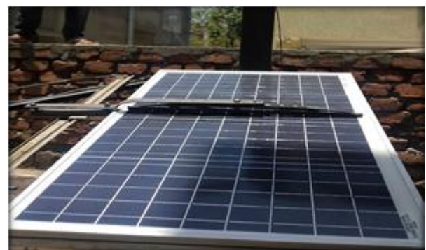
Fig. 3. Solar panel with cleaning mechanism.
