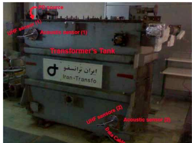
Fig 18. PD source (electrode) and sensor location.
