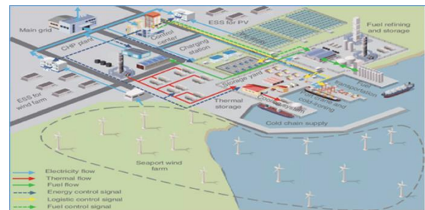
Fig. 5. Diagram of the Multi Energy Delivery System at a modern port [49].
