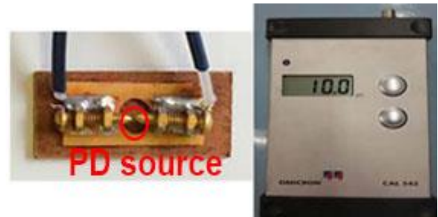
Fig. 16. PD source (electrode) & PD calibrator (set at 10 pC).
