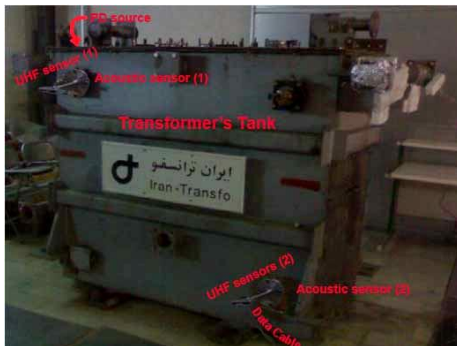
Fig. 18. PD source (electrode) and sensor location.
