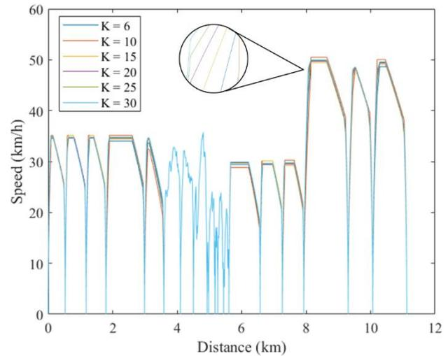
Fig. 10. Optimal speed profile of down track direction.
