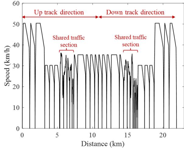
Fig. 6. Normal speed profile of round-trip.
