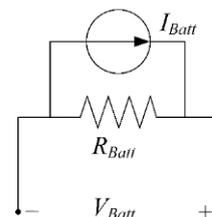
Fig. 2. Simplest battery model.
