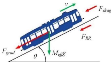
Fig. 1. Light rail vehicle movement model.
