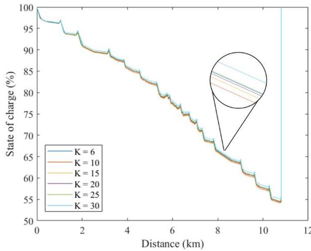
Fig. 9. State of charge of onboard battery of up track direction.
