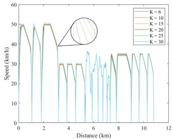
**Fig. 7. Optimal speed profile of up track direction.**
