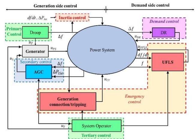
Fig. 1. The process of frequency control in power system.
