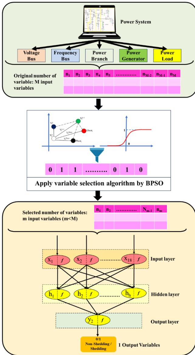
Fig. 5. Constructing Load Shedding Condition Recognition Model.
