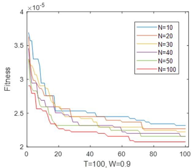
Fig. 6. Convergence characteristic of the BPSO variable selection algorithm execution.
