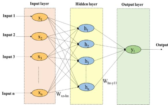
Fig. 2. Model of feedforward neural network.
