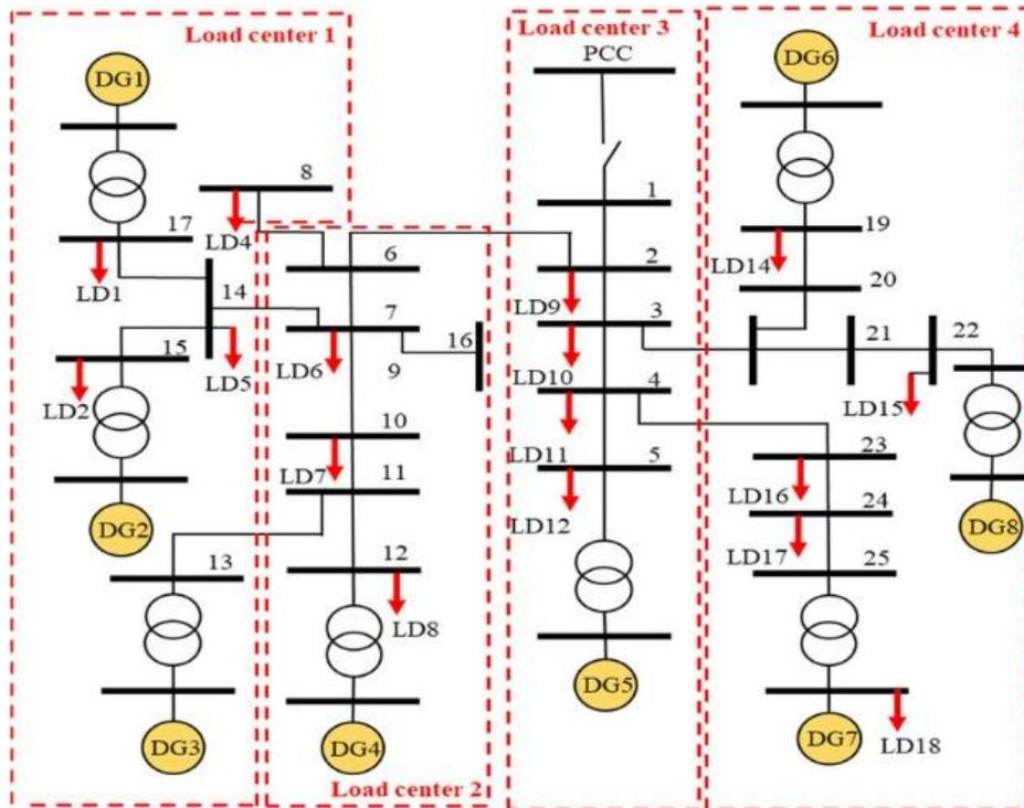
Fig. 4. IEEE 25 bus Microgrid diagram.
