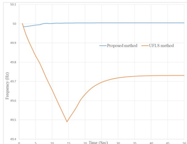
Fig 8. The recovery frequency values of 2 load shedding methods.
