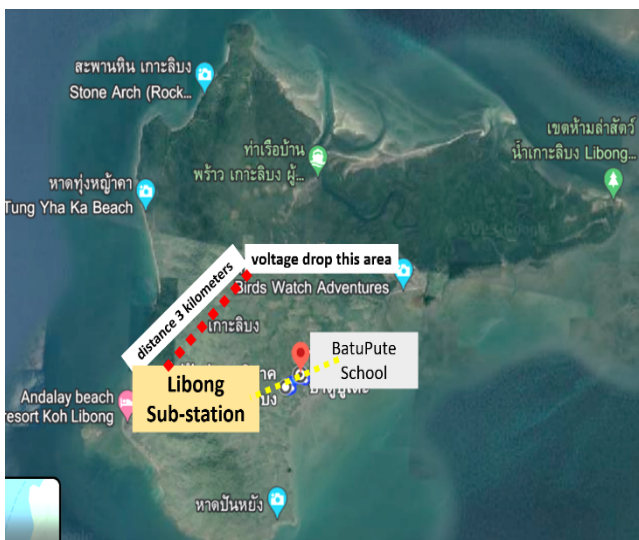
Fig. 14. Shows end-of-line areas and installation of photovoltaic systems.
